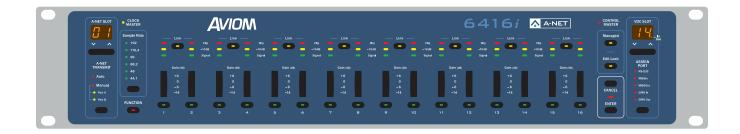
The 6416i Input Module provides 16 balanced line-level analog inputs to a Pro64<sup>™</sup> A-Net<sup>®</sup> network. Audio channels are converted to digital and inserted into the network.
