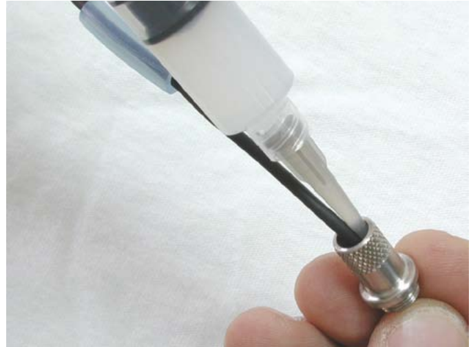
Figure 1 - Filling the Plug Cover with RTV
