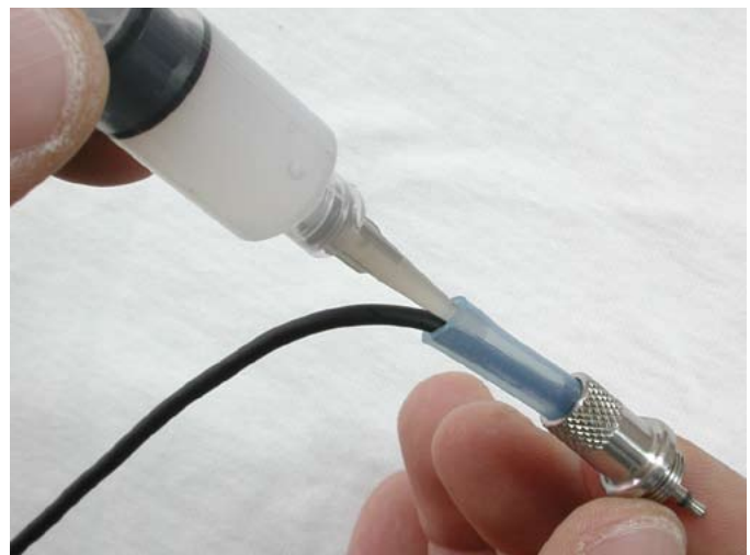
Figure 3 - Pulling the nozzle out as the tubing fills with sealant
