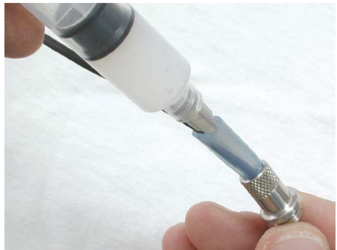
Figure 2 - Injecting the sealant deep into the tubing
