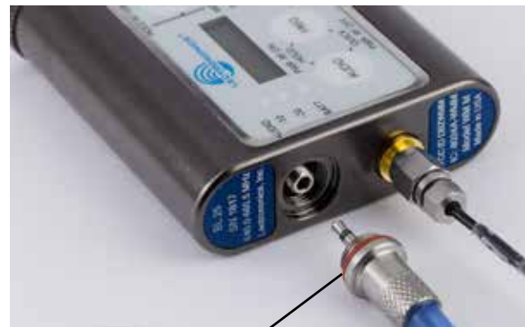
Treat O-ring with petroleum jelly before connecting (see page 18)
