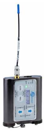
Designed for wet or dusty environments, the WM transmitter features O-ring sealed battery compartments and input jack, a compression sealed antenna port, and gasket sealed control panel and back cover. Dual AA batteries provide twice the operating time of earlier watertight transmitter designs. Larger membrane switches and control panel and a highly visible, backlit LCD enhance the user interface.
