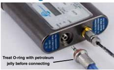
The threaded WP watertight plug on the microphone cable fits into a recessed jack on the top panel. The recess in the opening retains the O-ring when the plug is tightened. The Lectrosonics M152WP lavaliere microphone is supplied with the WP plug already installed. Other microphones can also be terminated with this plug by following the instructions included with the WP connector kits.
