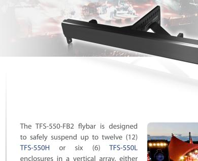
The TFS-550-FB2 flybar is designed to safely suspend up to twelve (12) TFS-550H or six (6) TFS-550L enclosures in a vertical array, either as unique or mixed arrays with a 10:1 safety factor. The flybar is secured to the uppermost speaker enclosure using the quick lock pins supplied with the cabinet, with additional enclosures attached in a similar manner below the previous element.
