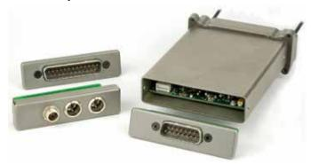
Power and audio connections are made through mating connectors on the adapter and receiver circuit boards.
