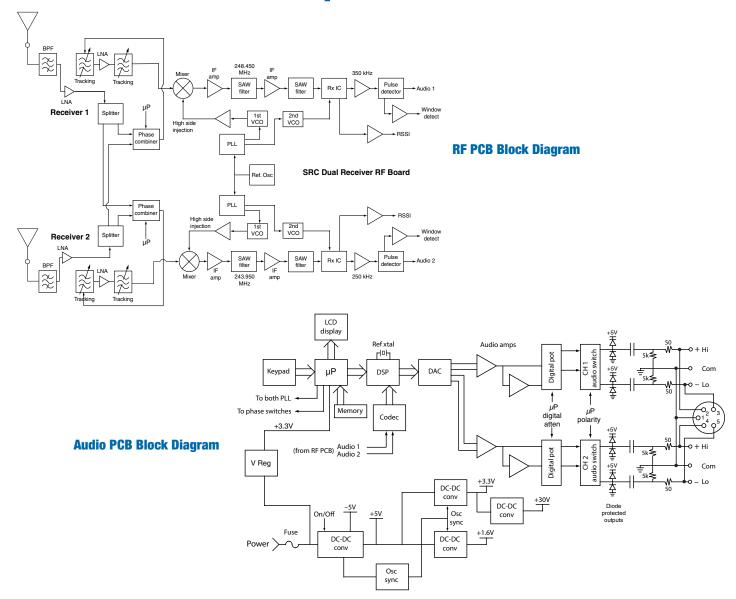
The design consists of two separate receivers built into a single, ultra compact housing with interchangeable adapters for video camera wireless receiver slots and stand-alone use. Digital Hybrid Wireless® technology provides superb, compandor-free audio quality and compatibility with other wireless systems. The RF performance is extremely stable over a very wide temperature range, making the receiver perfectly suited to the rough environmental conditions in field production.
