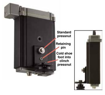
The clinch nuts in the foot and housing apply friction to the threads to allow the foot to be rotated to the desired position, with the jam nut locking it in place. Use a wrench to rotate the foot, then tighten the jam nut to prevent the foot from rotating.
