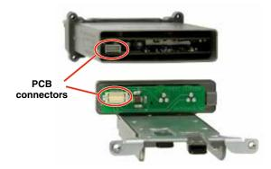
Slide the battery sled adapter into the end of the SR and gently seat it into place with the rear panel flush with the housing.
