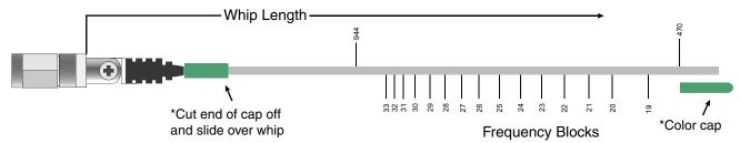
Trim the end of the color cap and slide the remaining sleeve over the whip - OR - Glue color cap onto the end
