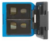
A pressure plate on the battery door compresses the battery contacts to maintain a solid connection with the batteries.
