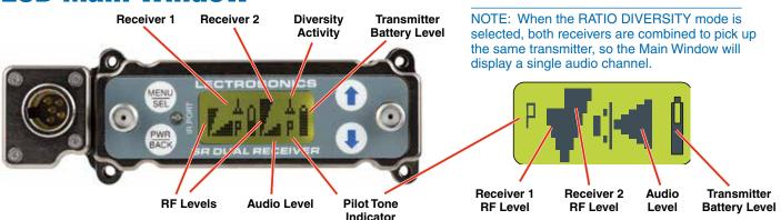
The Main Window displays information concerning the condition of the Pilot Tone, antenna phase, RF and audio signal levels and battery conditions for both the receiver and the associated transmitter.
