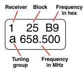
When any tuning mode other than NOR is selected, the frequency screen will include the selected tuning group number.
