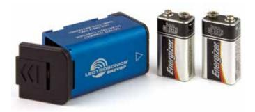
Slide the latch plate in the center of the door outward and swing the door open for access to two 9 volt battery compartments. Polarity barriers in each battery compartment protect against inserting the battery backwards. The circuitry is also protected electrically.
