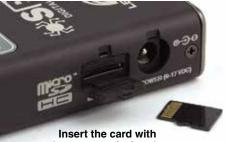
the contacts facing the control panel side of the recorder.
