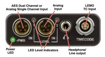
The audio input circuitry is essentially the same as on Lectrosonics SM and L Series transmitters. Any microphone wired as Lectrosonics "compatible" or "servo bias" will work with the SPDR.
