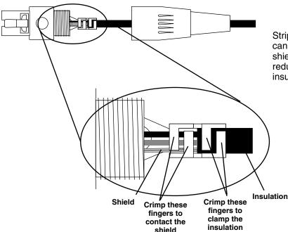
Strip and position the cable so that the clamp can be crimped to contact both the mic cable shield and the insulation. The shield contact reduces noise with some microphones and the insulation clamp increases ruggedness.
