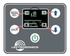
In Playback Mode, the soft buttons on the LCD change to provide the functions needed during playback. There are three variants of playback:
