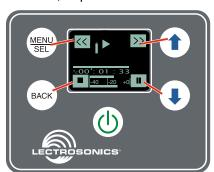
Press the keypad button next to each icon to operate the functions indicated by the soft buttons
