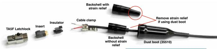
Note: If you use the dust boot, remove the rubber strain relief that is attached to the TA5F cap, or the boot will not fit over the assembly.
