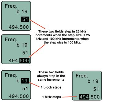
A fraction will appear next to the hex code in the setup screen and in the main window when the frequency ends in .025, .050 or .075 MHz.
