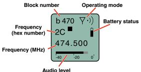
When the frequency step size is set to 25 kHz, the hex number will appear smaller and may include a fraction.
