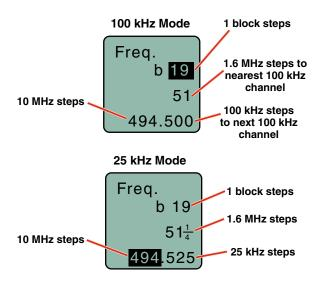
If the Step Size is 25 kHz with the frequency set between even 100 kHz steps and the Step Size is then changed to 100 kHz, the mismatch will cause the hex code to display as two asterisks.
