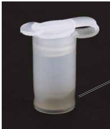
The tiny vial is about 1/2 inch tall and contains 25 mg of silver paste.
