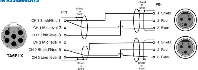
This cable is typically used to connect the output of a mixer or receiver with TA3M connectors to the line level input of a Lectrosonics transmitter with a TA6 connector. A common application is in a portable production bag system to connect the Lectrosonics Digital Camera Hop Transmitter.
