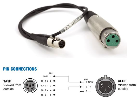
This cable is used to connect the AES output of a digital mixer or recorder to the AES input of the Lectrosonics SPDR portable recorder. It is constructed with a TA5F jack, rugged coaxial cable and a 3-pin female XLR connector. The connectors have soldered connections to the cable, allowing them to be serviced or replaced if the need arises.
