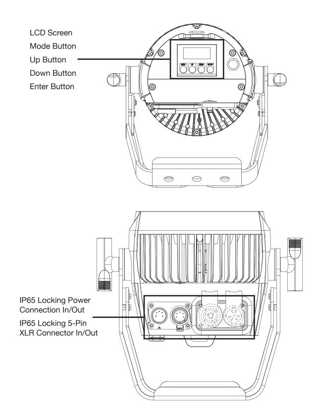
**DMX-512:** DMX is short for Digital Multiplex. This is a universal protocol used as a form of communication between intelligent fixtures and controllers. A DMX controller sends DMX data instructions from the controller to the fixture. DMX data is sent as serial data that travels from fixture to fixture via the DATA "IN" and DATA "OUT" XLR terminals located on all DMX fixtures (most controllers only have a DATA "OUT" terminal).
