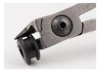
6. The grommet is needed if you are only mounting a single M2T unit into a rack, using the single rack mount kit (RMPM2T-1). Cut through the grommet so you can place it around the antenna cable.
