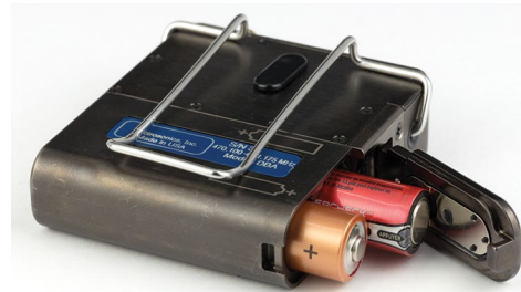
Battery compartment uses two AA batteries connected in series. Aluminum door latches securely.
