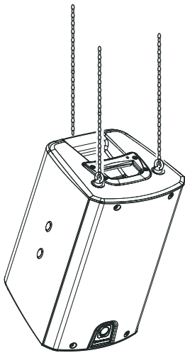
Suspension using M10 shoulder eyebolts.
