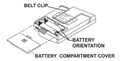
**NOTE:** If the unit is to be stored for any length of time be sure to remove the batteries from the unit.
