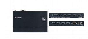
VA-4X is a versatile 4K@60Hz (4:4:4) HDMI multi-channel extender that equalizes and reclocks TMDS data before re-transmitting the signal, thus increasing the HDMI cable range for all 4 outputs. It is a true 4-channel HDMI "Toolbox", with functionality including 4 independent test-pattern generators, chroma sub-sampling down-conversion and EDID management options
