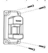
Fix the ball bracket to the rear of the loudspeaker using the supplied screws and a 3 mm Allen key. Two screws are used for AMS 5 models; four screws are used for AMS 6 and AMS 8 models.
