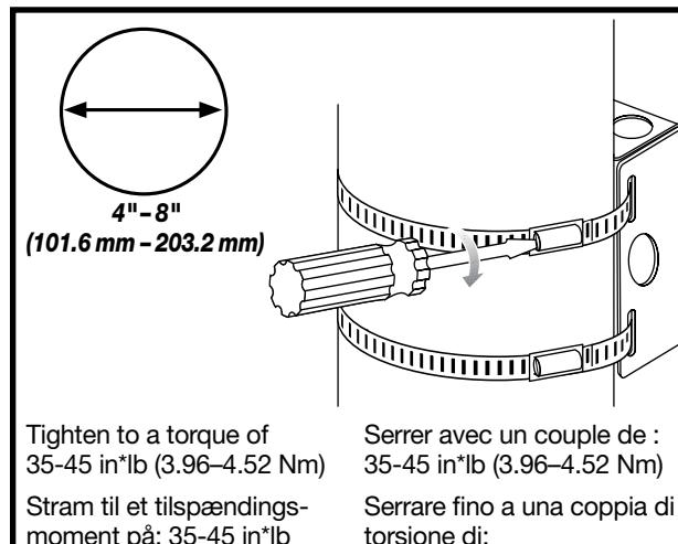
Tighten to a torque of
