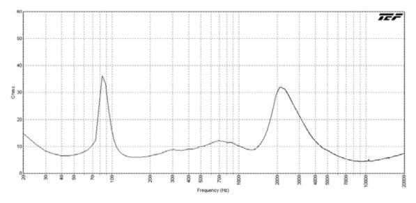
AH94-12T-BSG Impedance (Ohms) vs. Frequency
