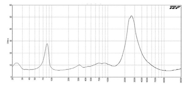
AH66-12T-BSG Impedance (ohms) vs. Frequency
