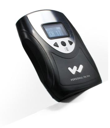
The newest addition to the Personal PA FM line - the stylish, new PPA SelectView™ FM receiver - is easy on the eyes and convenient to use. The high-res OLED screen presents a quick view of receiver status and immediate access to all user settings. The highlight: on-screen channel selection with easy access to 17 pre-set, wideband frequencies (72-76 MHz).
