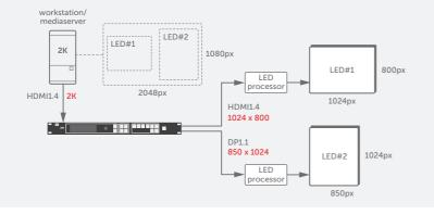
Dual outputs feeding two LED walls from the same content server. Outputs can be sized, positioned, and configured independently.\*
