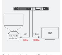
Dual output feeding an HD projector and a monitor, both independently scaled.\*
