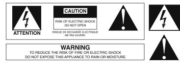
The lightning flash with arrowhead symbol within an equilateral triangle, is intended to alert the user to the presence of uninsulated "dangerous voltage " within the product's enclosure that may be of sufficient magnitude to constitute a risk of electric shock to persons.
