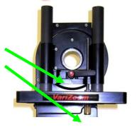
the platform to precisely raise or lower it – you can use a hex key. Try to get the center of mass right on the center of tilt rotation. Rotate the platform to various angles and adjust until it holds position at any angle. If it falls down, you need to adjust the platform upward. If it drifts upward, you need to lower the platform. When balance is achieved, tighten the platform locking lever.
