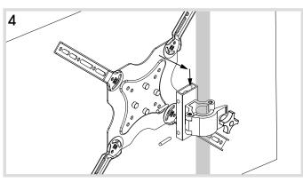
Attach the display with VESA mount to the pole mount by aligning the keyhole studs with the key holes on the pole mount then insert safety pins.
