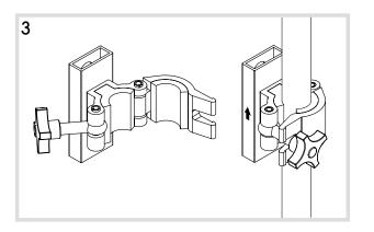
Attach the pole mount to a 35mm-38mm diameter pole, and hand tighten until secure. (Arrow points up)
