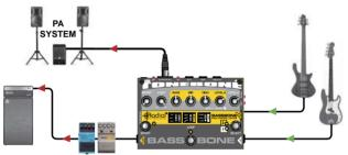
To take things one step further, the Bassbone is equipped with an unique effects loop designed specially for bass. The effects loop lets you insert pedals by depressing a footswitch and mix the effects with the original bass signal to preserve the fundamental tone of your bass. You can also assign the effects loop to channel-1, channel-2 or both, giving you absolute freedom. Connected this way, the pedals will be heard through your amp and in the PA system.
