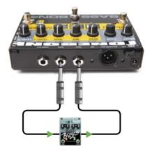
Depress the LOOP footswitch to turn the function on, the LED indicator will illuminate. *Note: If there are no pedals connected to the SEND and RECV jacks the LOOP footswitch will have no effect on the sound. You cannot accidentally mute your sound because there are no pedals connected.*
