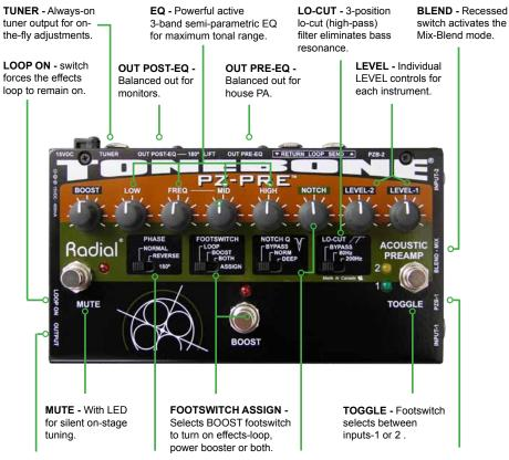
**OUTPUT -** For the on-stage instrument amp.
