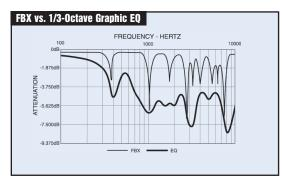
A PA System was set up using a microphone, mixer, FBX, power amp and two speakers. The system's gain was raised until the FBX removed nine feedback points. Next the FBX was replaced with a graphic EQ. The EQ was adjusted while the system gain was raised to the same level achieved with the FBX. The frequency response curves of each device were then plotted.
