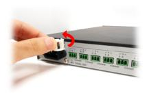
**Step3.** Wire the 3pin removable terminal plug which is supplied with N-8000/8010RS, and insert it into the terminal block on the Q-N8000LC. The other end of this wire connects to the corresponding device.
