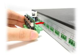
**Note:** When mounting on ports 1 through 4, please lift up the cable clamp as shown below.
