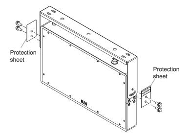
**Step 2.** Secure the mounting bracket to the installation location.
