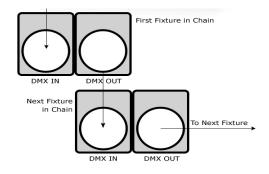
of a (male) 3-pin connector. Then, proceed to connect from the output as stated above to the input of the following fixture and so on.
