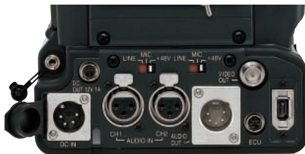
AJ-SPX800 Rear Connector Panel
