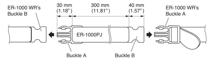
Step 1. Insert ER-1000PJ's Buckle A into ER-1000 WR's Buckle B until it clicks into place.
