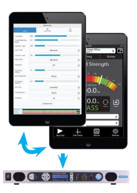
Loopworks<sup>™</sup> Measure App with LoopLink also enables you to remotely control the test signals of a connected Ampetronic C or D Series driver, change the settings via the drivers web app and see the results in the performance of the magnetic field instantly without repeated journeys between the amplifier and looped area.
