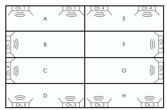
Diagram 2. Single channel air wall system using auto-seek, 8 room air wall system with all air walls CLOSED.
