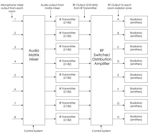
Diagram 4. Single channel air wall system using RF switcher/distribution amplifier
