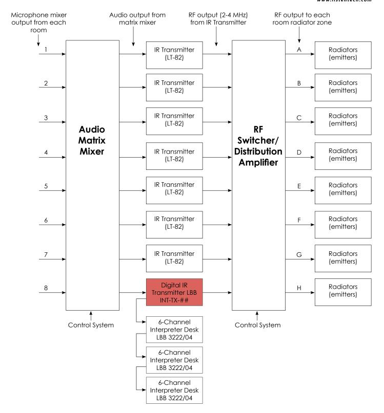
Diagram 9. Multiple channel system with 4 to 32 channels of language interpretation using Listen Stationary IR and Digital IR transmitters and receivers.
