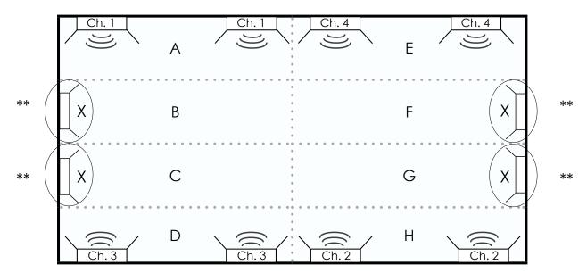
Diagram 3. Single channel air wall system using auto-seek, 8 room air wall system with all air walls OPEN.
