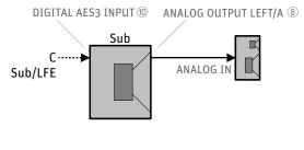
Source Signal: Analog Subwoofer-loudspeaker connections: Digital Source Signal: Digital Subwoofer-loudspeaker connections: Digital
