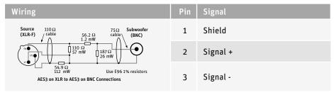
This method brings impedance matching and level matching, but no source-receiver isolation. Use a resistor network to passively attenuate the XLR signal from 3.1 V down to 0.42 V and change the impedance from 110  $\Omega$  to 75  $\Omega$ .
