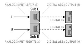
Note: Set the left loudspeaker input signal select to Digital A and the right loudspeaker input signal select to digital B.
