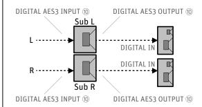
Note: Set the left loudspeaker input signal select to Digital A and the right loudspeaker input signal select to digital B.
