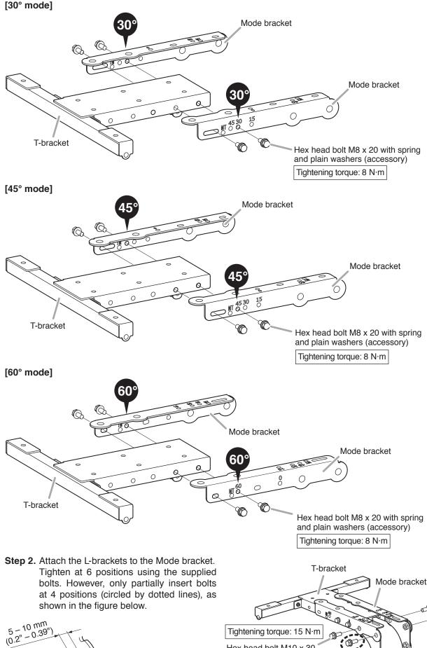
Partially insert the bolt with a gap as illustrated.
