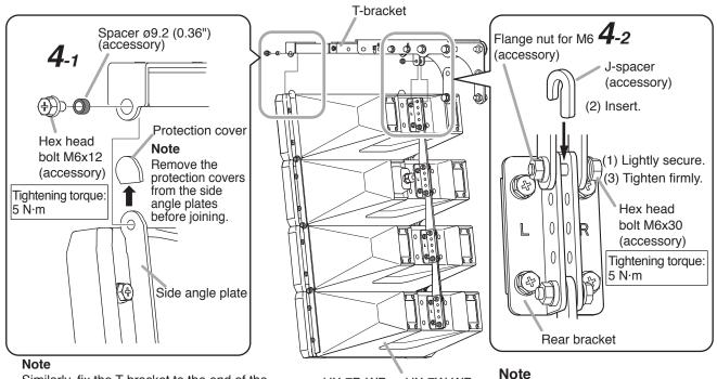
Similarly, fix the T-bracket to the end of the side angle plate on the opposite side.
