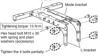
Step 3. (When mounting the MT-200 Matching transformer)<br/>Mount the MT-200 to the mode bracket.<br/>Use the supplied bolts and nuts to mount, as<br/>shown in the figure at right.Hex head<br/>spring and<br/>(MT-200's<br/>Tightening<br/>8 N·mFor MT-200 wiring, refer to the instruction<br/>manuals supplied with the MT-200 and the<br/>HX-7 Series speaker.Tightening<br/>8 N·m
