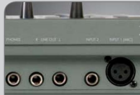
Audio inputs include one XLR with phantom power
