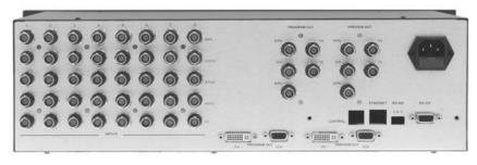
The VP-727 In-CTRL™ Dual Scaler Seamless Switcher is a true multi-standard video to graphics scaler and seamless switcher with 8 universal inputs comprised of 5 BNCs each of which can accommodate a composite video, s-Video (Y/C), component video (RGB/YUV), RGBS, or RGBHV signal. It has dual scalers, one for the preview and the other for the program output. Dual scalers are required to do "live" seamless transitions from one source to another.
