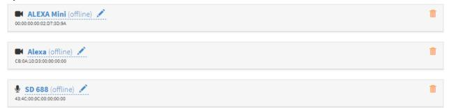
The MasterLockit will preserve previous connected cameras and sound recorders for convenient reconnection. In case you want to remove those without a complete reset, you can delete them here.
