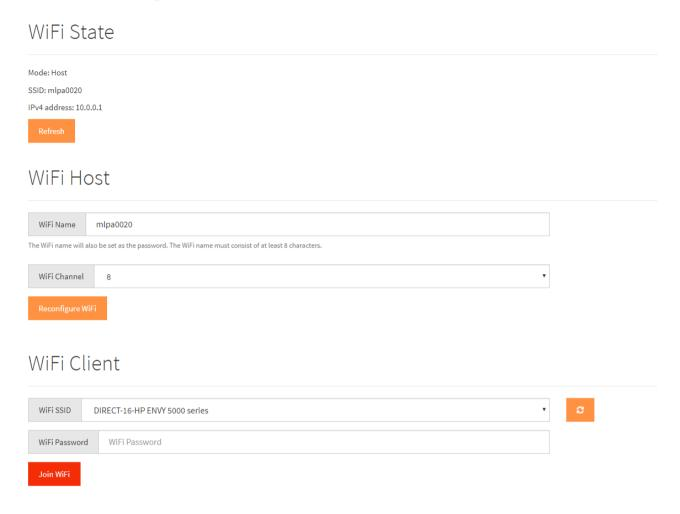
Shows info of the current WiFi configuration. When running as host you can rename WiFi SSID and change the channel. After hitting reconfigure WiFi, the MasterLockit will immediately apply the new **SSID** so you will lose connection and need to log in again with new credentials.
