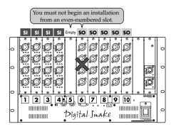
Modules of a different type cannot be installed even-numbered slots first. SI SO SO Ö ø Ø ø Ø Ø 9|9|9 ø 1 2 3 4 Digital Snake 1111111111111 |SI| = SI-AD4
