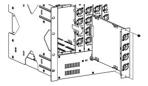
Remove the two screws from each module (SI-AD4 or SO-DA4) installed in the S-4000S.
