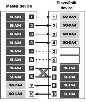
The audio input into the Master device is transmitted to the modules on the connected device (a Slave device or the like).
