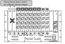
■ The modules installed in a device serving as the counterpart to a device for which the REAC mode is Master need to be of a different type.
