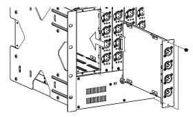
Align the module's circuit board with the slot in the S-4000S, and insert slowly.
