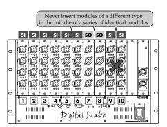
■ On a device for which the **REAC** mode is Master, be sure to install modules in slots 1 and 2.
