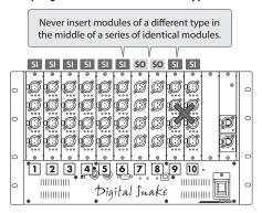
• On a device for which the REAC mode is Master, be sure to install modules in slots 1 and 2.
