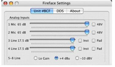
via the rotary encoder, or via the Settings dialog. The current gain is displayed in dB left to the fader. Further information is found in chapter 27.3.
