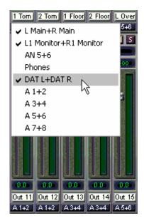
The hardware outputs (third row) can be edited in the same way. In this case, the names in the routing drop down menus will change automatically. Additionally the names in the drop down menus of the Monitor section will change as well.
