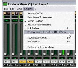
After a mouse click TotalMix sets gains and pans correctly. Of course these settings can also be performed manually. Repeat the last step to remove all routings (*menu Options ...Off*).
