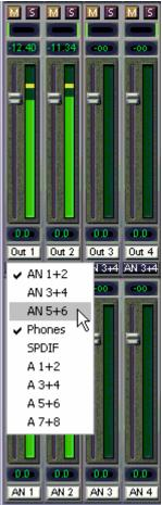
Please set Out 4 to a gain of around -20 dB and the pan close to center. Now click onto the routing field. You'll now see two checkmarks, one at 'AN 3+4', the other one at 'AN 5+6'. Click onto 'SPDIF'. The window disappears, fader and pan jump to their initial values, the signal can now be routed to the SPDIF output. You can continue like this until all entries have got a checkmark, i. e. you can send the signal to all outputs simultaneously.
