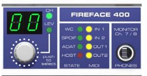
**Phones** is a low impedance line output of highest quality. It provides a sufficient and undistorted volume even when used with headphones.
