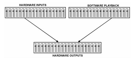
36 channels don't fit on the screen side by side, neither does such an arrangement provide a useful overview. The input channel should be placed above the corresponding output channel. Therefore, the channels have been arranged as known from an *Inline* desk, so that the row *Software Playback* equals the *Tape Return* of a real mixing desk:
