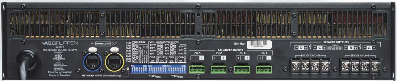
NomadLink® network In/Out on RJ45 Gain, Bridge mode, Voltage Peak Limiter Phoenix connector input Screw terminals output
