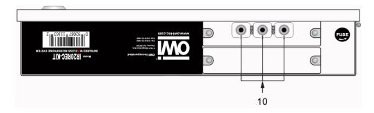
Figure 5. IR20REC-CASE Top Side Panel
