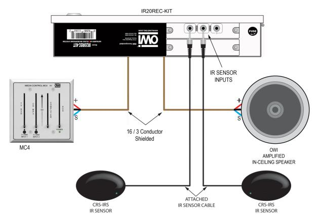
Figure 14. Typical CRS System Connections
