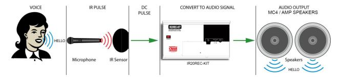
Figure 15. IR20REC-KIT System Signal Path
