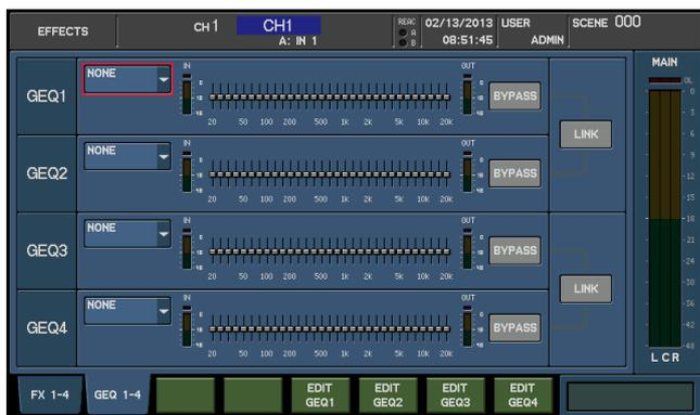
2. Move the cursor to the LINK button located at the right of GEQ1 and GEQ2, and press [ENTER] to turn the button on.
