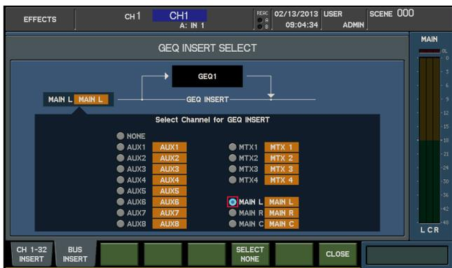
4. Move the cursor to the MAIN L insert-destination channel select button, and press [ENTER] to select it.
