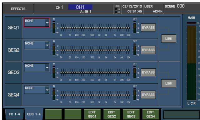
2. Move the cursor to the GEQ INSERT SELECT popup button for the desired GEQ, and press [ENTER].
