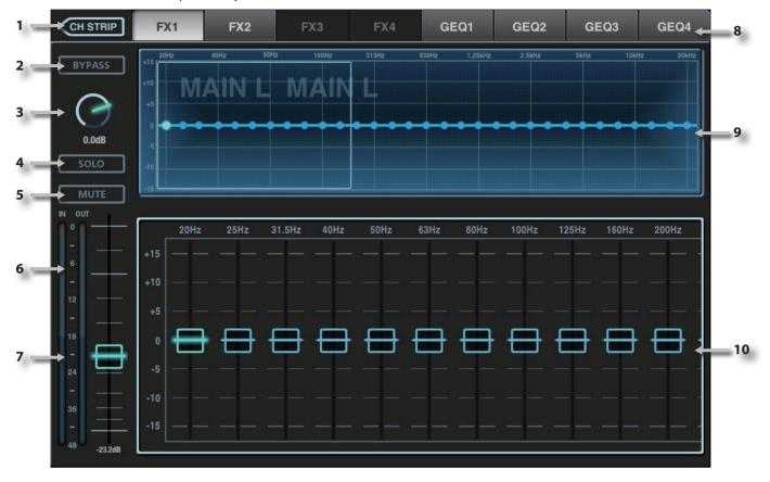
The GEQ button on the side panel lets you access the GEQ screen on the main section.
