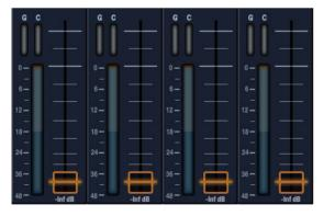
The color of faders will change according to the label of the target bus.
