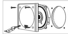
Both the M5CX and M4F weatherized speakers are held in place by (4) #8 stainless steel screws. Locate the speaker grill covers and put a small amount of silicone in screw holes. This will seal the screws. Using the Philips screw driver, install the (4) #8 screws carefully aligning speaker in wall. (It is not necessary to seal the speaker grill cover - only the screw holes.)
