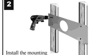
frame A on the wall using screw or staple.
