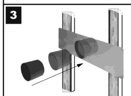
Place cup B on the hole of the mounting frame A.
